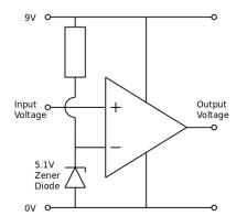
The zener diode in reverse bias and the series resistor provide a fixed voltage at the inverting input of the operational amplifier. In the diagram, this is 5.1V.
