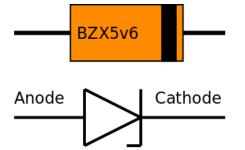
Zener diodes can be identified by the letter "Z" in the name or by having the zener voltage as part of the name. For example a 1N4148 is a regular silicon diode whereas a BZX85c5v6 is a zener diode with a zener voltage of 5.6 volts. In the image of zener diodes the blue and red examples are labelled 5v1 and the smaller orange one is labelled BZX.
