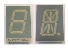
The 7 segment display is an arrangement of 7 LEDs and a separate LED for the decimal place. The display can form the digits 0-9 to display decimal numbers and can
