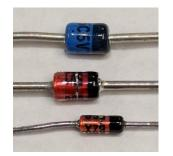
The zener voltage is a characteristic of a zener diode. Any given zener diode has a very specific fixed zener voltage. Zener diodes are available in many different zener voltages ranging from 1.8 V up to voltages in excess of 100 V.
