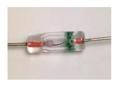
When we talk about a diode we are almost invariably talking about a silicon diode. Diodes are also made from a semiconductor called Germanium. A Germanium diode has a very low forward bias potential difference of around 0.1V making them ideal for use in very low voltage circuits.
