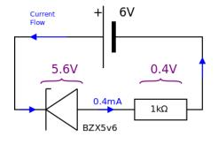
When the cathode is connected to the battery positive the zener diode is reverse biased. The battery voltage is greater than the zener voltage (5.6V) and so the zener diode conducts. The voltage drop across the zener diode is maintained at 5.6V and the potential difference across the  $1\,k\Omega$  resistor is therefore 0.4V leading to a circuit current of 0.4 mA.
