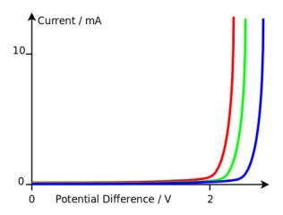
LEDs do not conduct when reverse biased and so the current in zero, the LED is not illuminated.
