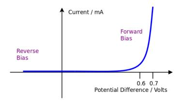
In reverse bias the current remains zero even when the potential difference increases to several volts.
