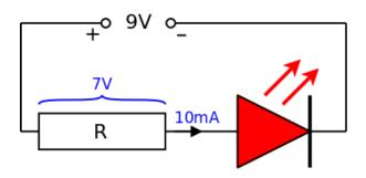
All LEDs have a different forward bias voltage and a different optimal current.
