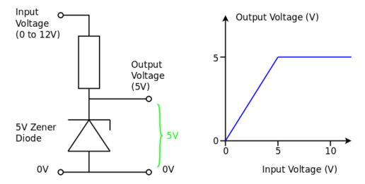
When the potential difference across the zener diode is less than the zener voltage no current flow through the zener diode. Assuming no current flows through the load, the potential difference across the resistor will be zero and the output voltage is the same as the input voltage. If current flows through the load, the output voltage will be less than the input voltage due to the potential difference across the resistor.
