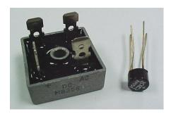
A diode, or several diodes, can be used to convert A.C. into D.C. by only allowing current to flow in one direction. Rectifier diodes can usually handle large forward bias currents and have a reverse breakdown voltage greater than the peak voltage of the A.C. being rectified.
