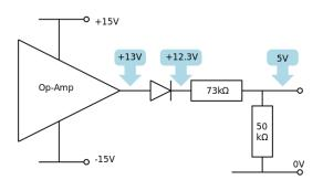
When the output from the comparator is +13V the diode is forward biased and conducts. The potential divider is used to create a 5V Logic signal (Logic 1). The voltage drop across the diode is 0.7V and so the potential divider must reduce 12.3V to 5V.
