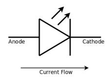
The humble LED used in school electronics comes in many shapes and sizes but, most commonly, they are circular with a diameter of 5 mm and come in a range of colours from Red to Blue.
