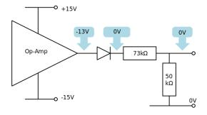
The potential difference across the two resistors are in the ratio 7.3:5 and therefore a  $73\,k\Omega$  and a  $50\,k\Omega$  resistor are used. In reality values from the E24 series such as  $68\,k\Omega$  and  $47\,k\Omega$  would be used.
