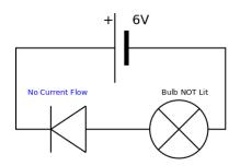
No current flows in the circuit and the potential difference across the bulb is 0 V. Therefore, the (reverse) potential difference across the diode is 6 V. If the reverse bias voltage is too high the diode will be damaged. All diodes have a maximum reverse bias voltage.
