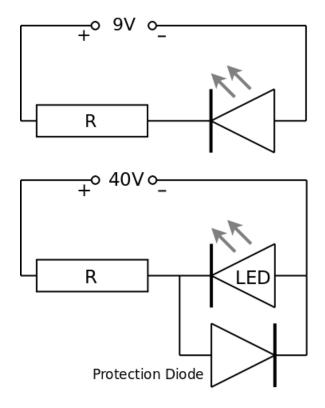
In reverse bias, current cannot flow from the cathode to the anode and the LED does not light.
