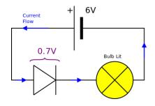
In this example the forward bias voltage across the diode is 0.7V and the potential difference across the bulb is 5.3V.
