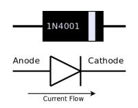
A diode has two leads called the anode and the cathode and current can only flow from the anode to the cathode.
