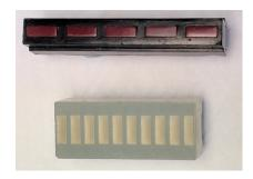
An LED array is simply a series of individual LEDs packaged together to make a single display unit. The LEDs are all electrically separate and each element of the array requires a series resistor. These are useful for bar graphs and VU meters as well as being used to make futuristic looking machines in old school Si-Fi movies.
