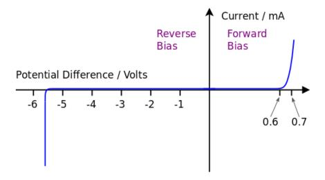
In forward bias the current is initially zero when the potential difference is less than 0.6V and then the current rapidly increases as the potential difference increases to from 0.6V to 0.7V. The forward bias potential difference does not exceed much more than 0.7V when current flows through the zener diode and therefore the zener diode is used in series with other components.
