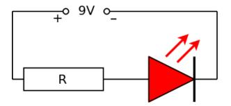
An LED is forward biased when current can flow from the anode to the cathode.
