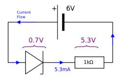
When the anode is connected to the battery positive the zener diode is forward biased and it behaves in the same way as a silicon diode.
