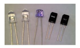
Infrared (IR) LEDs are exactly like regular LEDs except that they do not emit visible light. This makes them harder to test therefore a multimeter must be used.
