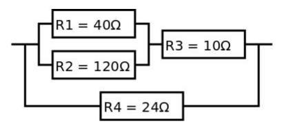
In this more complex example the resistors must once again be combined in pairs in the correct order. First R1 and R2 are added in parallel. Next the series resistor R3 is added to the previous result. Finally the total of R1, R2 and R3 is added in parallel to R4 ... simple!
