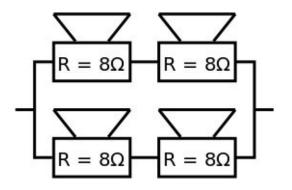
The diagram shows how this is accomplished. The two  $8\Omega$  speakers in series add up to  $16\Omega$ . The two  $16\Omega$  pairs in parallel make  $8\Omega$  in total.
